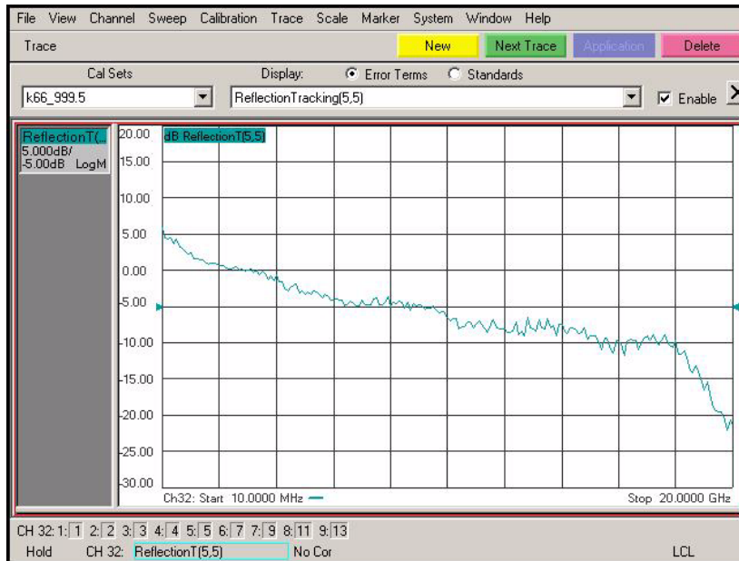
Figure 27 Port 5 and 6 Reflection Tracking Trace
